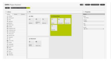
3. Creating a building: The desired building is created quickly and easily using drag & drop. Devices and functions can be located in the same manner.
